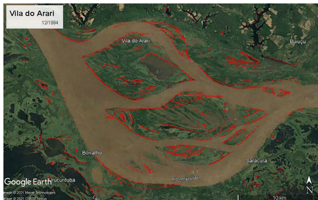
Figure 9 - Erosion polygons (red lines) in a 1984 (December) Landsat image of Arari Village (Amazon River).
