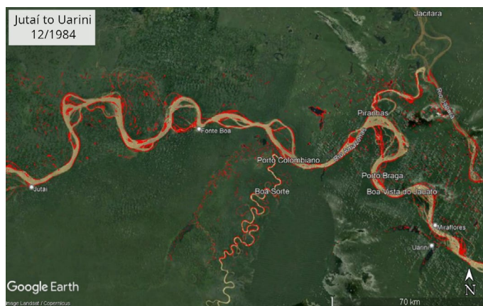
Figure 2 - Erosion polygons of Area 1 (Solimões River) in December 1984 (1a). the red areas are the ones that would be eroded up to 2018.
