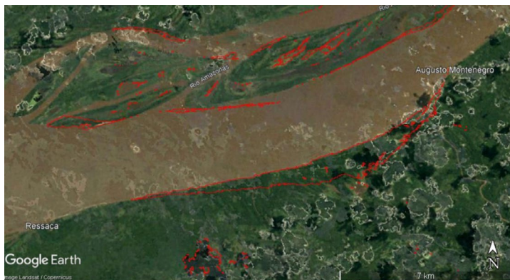
Figure 7 - Erosion polygons (red lines) in a 1984 (December) Landsat image of the region near Augusto Montenegro (Amazon River).
