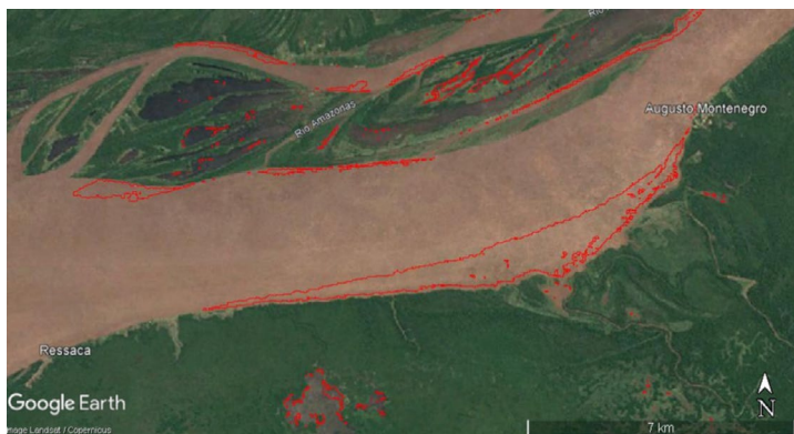
Figure 8 - Erosion polygon (red lines) in a 2020 (December) Landsat image of the region near Augusto Montenegro (Amazon River).
