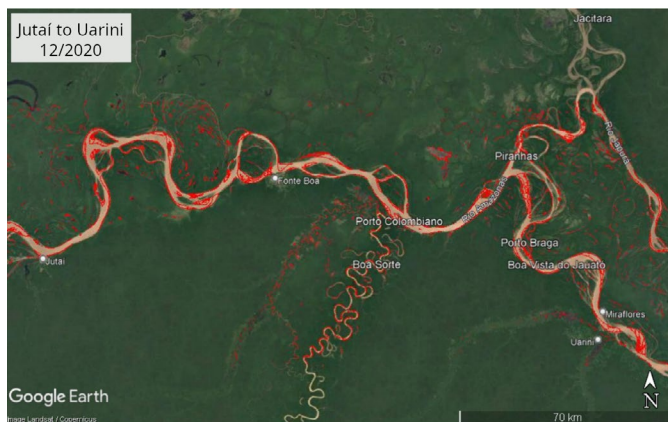
Figure 3 - Erosion polygons of Area 1 in December 2020 (1b). The red areas are the ones that have been eroded up to 2018.
